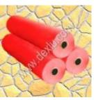
Prepreg DMD is formed in the process of precuring the modified F-class DMD with Impregnation of hi-temp resistant B-stage Epoxy resin by baking. With long shelf life at room temp, low precuring temp & time, excellent electrical insulation, bonding and heat-resistant properties. Its thermal Glass is F, widely used for liner insulation of copper foil (aluminum foil)-wrapped Low voltage coils in dry-type transformer and slot insulation & phase insulation in B~F class Motor & electrical appliances.
